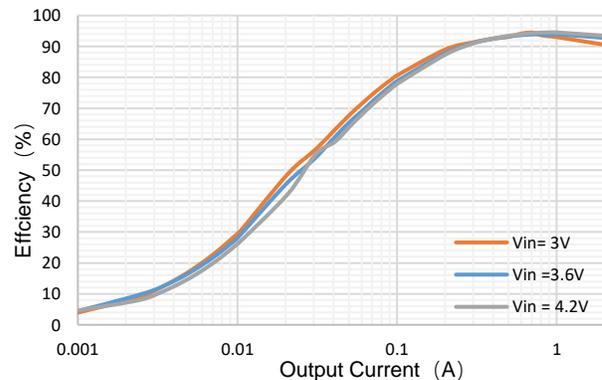
Efficiency vs Load Current, Vout=9V
