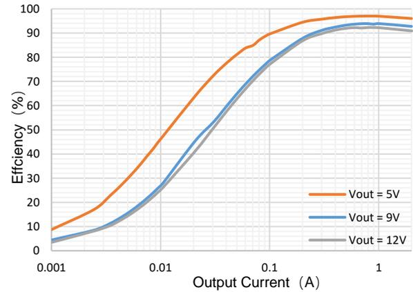
Figure 2. SCT1270F Efficiency vs Load Current, Vin=3.6V
