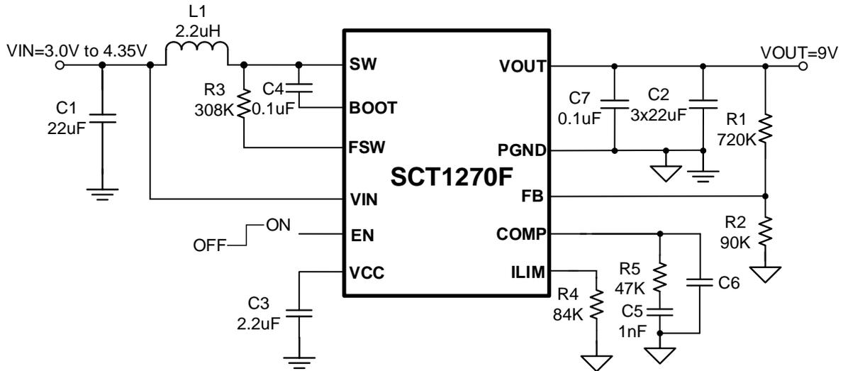
Figure 8. One Cell Battery Input, 9V/2A (20W) Output
