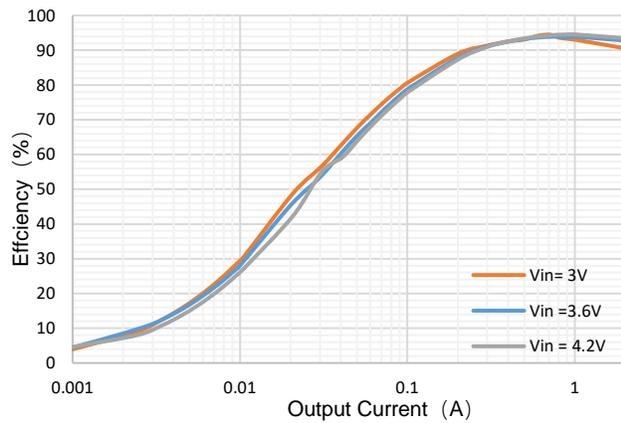
Figure 1. SCT1270F Efficiency vs Load Current, Vout=9V
